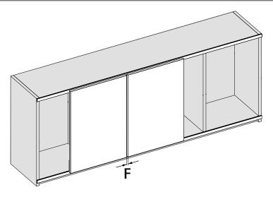
The centre reveal F between two wooden doors can be influenced by the position of drill holes B1 and B2 for the running and guide components. Use of the standard drilling pattern produces a centre reveal of F = 10 mm
